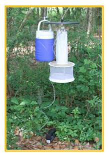
**Dry Ice Traps** are designed to collect host seeking nuisance mosquitoes, particularly Tiger Mosquitoes, *Aedes albopictus*, and a variety of floodwater species. A thermal container holds solid carbon dioxide pellets that slowly sublimate. The insects are attracted to the CO2, just as they are attracted to exhaling humans and animals. The mosquitoes are pulled into the net by a battery-operated fan.
